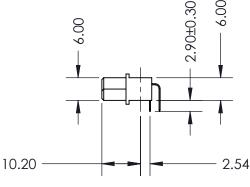
Dimension E at 2.54 Pitch: E= No. of Positions-1 X 2.54 E= (No. of Positions/2)-1 X 2.54
