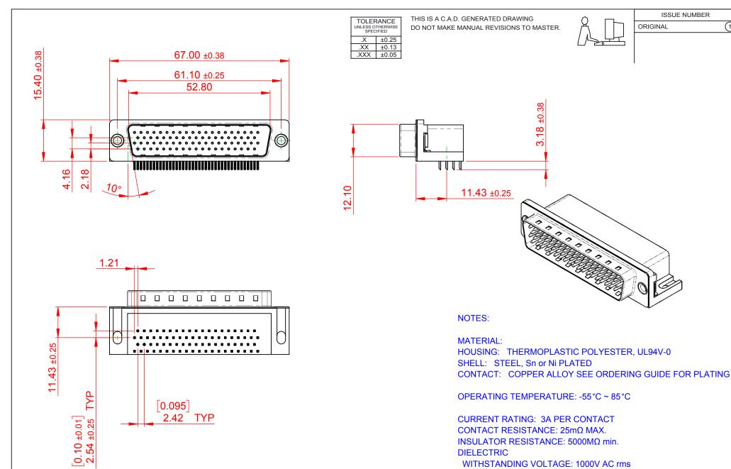
WITHSTANDING VOLTAGE: 1000V AC rms
