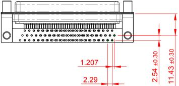
HOUSING: PA6T, UL94V-0 SHELL: STEEL, Sn or Ni PLATED CONTACT: PRECISION MACHINED COPPER ALLOY SEE ORDERING GUIDE FOR CONTACT PLATING
