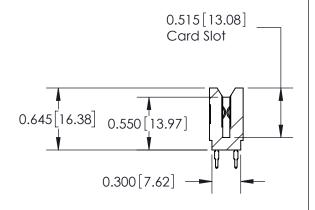
737 Series Ultra-Mate Card Edge Connector - Press Fit Part Number: 737-010-520-206
