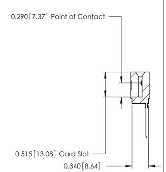
ACAD REFERENCE NO. 746-ENG MASTER 746 Series Ultra-Mate Card Edge Connector - Press Fit DRAWN: J.LEE DATE: AUG 20/09 Part Number: 746-006-553-101 CHECKED: DATE: **EDAC INC** SCALE: SHEET 1 OF 1 THESE DRAWINGS AND SPECIFICATIONS ARE THE PROPERTY OF EDAC INC.,AND TORONTO, ONTARIO SHALL NOT BE REPRODUCED, OR COPIED DRAWING NUMBER CANADA OR USED AS THE BASIS FOR THE 746-ENG MASTER MANUFACTURE OR SALE OF APPARATUS YOUR CONNECTION TO QUALITY & SERVICE WITHOUT WRITTEN PERMISSION.
