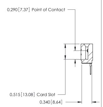
ACAD REFERENCE NO. 746-ENG MASTER 746 Series Ultra-Mate Card Edge Connector - Press Fit DRAWN: J.LEE DATE: AUG 20/09 Part Number: 746-009-527-101 CHECKED: DATE: **EDAC INC** SCALE: SHEET 1 OF 1 THESE DRAWINGS AND SPECIFICATIONS ARE THE PROPERTY OF EDAC INC.,AND TORONTO, ONTARIO SHALL NOT BE REPRODUCED, OR COPIED DRAWING NUMBER CANADA OR USED AS THE BASIS FOR THE 746-ENG MASTER MANUFACTURE OR SALE OF APPARATUS YOUR CONNECTION TO QUALITY & SERVICE WITHOUT WRITTEN PERMISSION.
