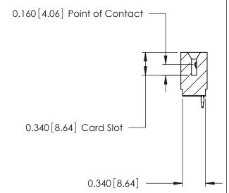
ACAD REFERENCE NO. 746-ENG MASTER 746 Series Ultra-Mate Card Edge Connector - Press Fit DRAWN: J.LEE DATE: AUG 20/09 Part Number: 746-011-525-501 CHECKED: DATE: **EDAC INC** SCALE: SHEET 1 OF 1 THESE DRAWINGS AND SPECIFICATIONS ARE THE PROPERTY OF EDAC INC.,AND TORONTO, ONTARIO SHALL NOT BE REPRODUCED, OR COPIED DRAWING NUMBER **ISSUE** CANADA OR USED AS THE BASIS FOR THE 746-ENG MASTER MANUFACTURE OR SALE OF APPARATUS YOUR CONNECTION TO QUALITY & SERVICE WITHOUT WRITTEN PERMISSION.
