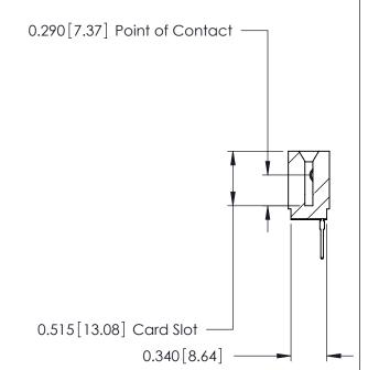
ACAD REFERENCE NO. 746 Series Ultra-Mate Card Edge Connector - Press Fit DRAWN: J.LEE Part Number: 746-012-527-101 CHECKED: **EDAC INC** SCALE: THESE DRAWINGS AND SPECIFICATIONS ARE THE PROPERTY OF EDAC INC.,AND TORONTO, ONTARIO SHALL NOT BE REPRODUCED, OR COPIED DRAWING NUMBER CANADA OR USED AS THE BASIS FOR THE 746-ENG MASTER MANUFACTURE OR SALE OF APPARATUS YOUR CONNECTION TO QUALITY & SERVICE WITHOUT WRITTEN PERMISSION.
