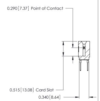
ACAD REFERENCE NO. 746-ENG MASTER 746 Series Ultra-Mate Card Edge Connector - Press Fit DRAWN: DATE: AUG 20/09 J.LEE Part Number: 746-012-527-201 CHECKED: DATE: **EDAC INC** SCALE: SHEET 1 OF 1 THESE DRAWINGS AND SPECIFICATIONS ARE THE PROPERTY OF EDAC INC.,AND TORONTO, ONTARIO SHALL NOT BE REPRODUCED, OR COPIED DRAWING NUMBER CANADA OR USED AS THE BASIS FOR THE 746-ENG MASTER MANUFACTURE OR SALE OF APPARATUS YOUR CONNECTION TO QUALITY & SERVICE WITHOUT WRITTEN PERMISSION.
