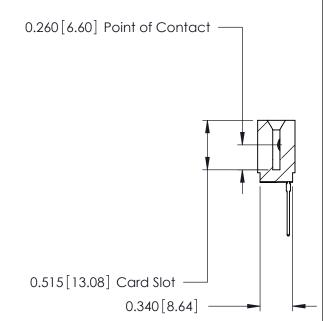
ACAD REFERENCE NO. 746-ENG MASTER 746 Series Ultra-Mate Card Edge Connector - Press Fit DRAWN: J.LEE DATE: AUG 20/09 Part Number: 746-012-540-101 CHECKED: DATE: **EDAC INC** SCALE: SHEET 1 OF 1 THESE DRAWINGS AND SPECIFICATIONS ARE THE PROPERTY OF EDAC INC., AND TORONTO, ONTARIO SHALL NOT BE REPRODUCED, OR COPIED DRAWING NUMBER **ISSUE** CANADA OR USED AS THE BASIS FOR THE 746-ENG MASTER MANUFACTURE OR SALE OF APPARATUS YOUR CONNECTION TO QUALITY & SERVICE WITHOUT WRITTEN PERMISSION.
