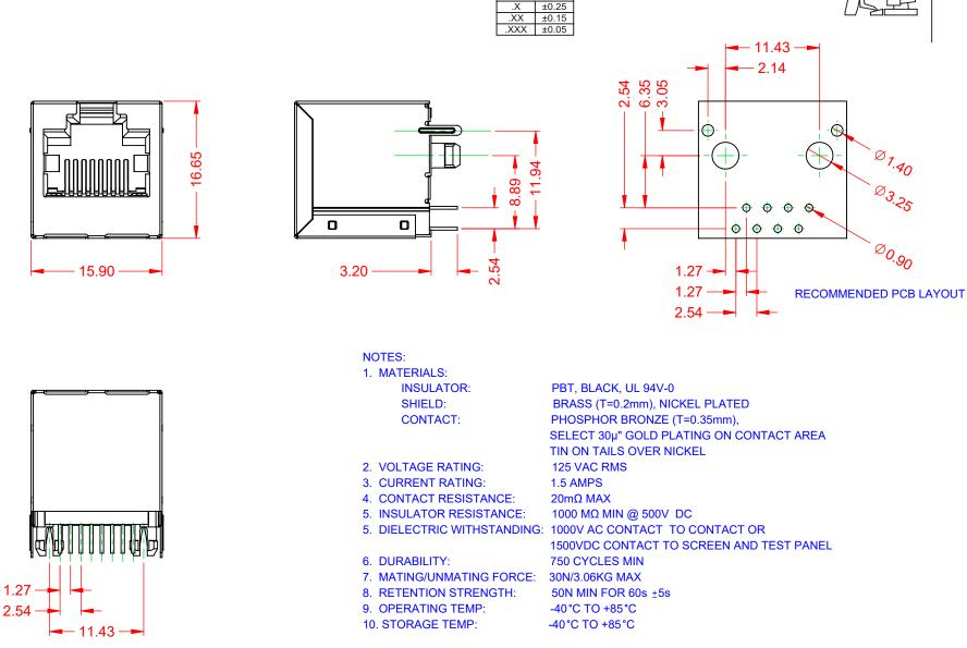
MATES WITH MODULAR PLUG CONFORMING TO FCC PART 68, SUBPART F.
