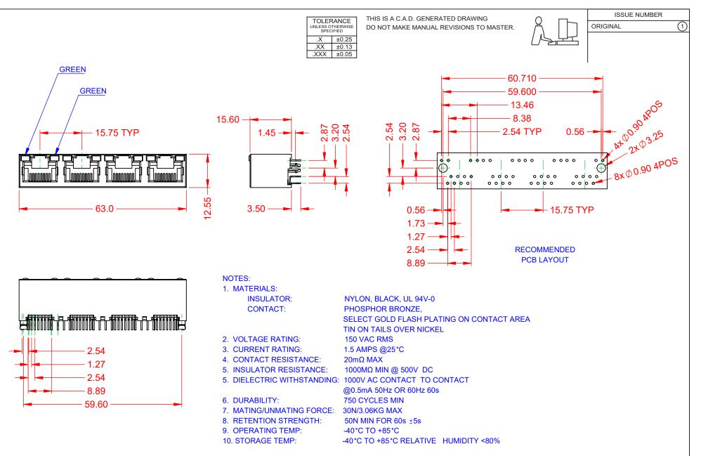
MATES WITH MODULAR PLUG CONFORMING TO FCC PART 68, SUBPART F.
