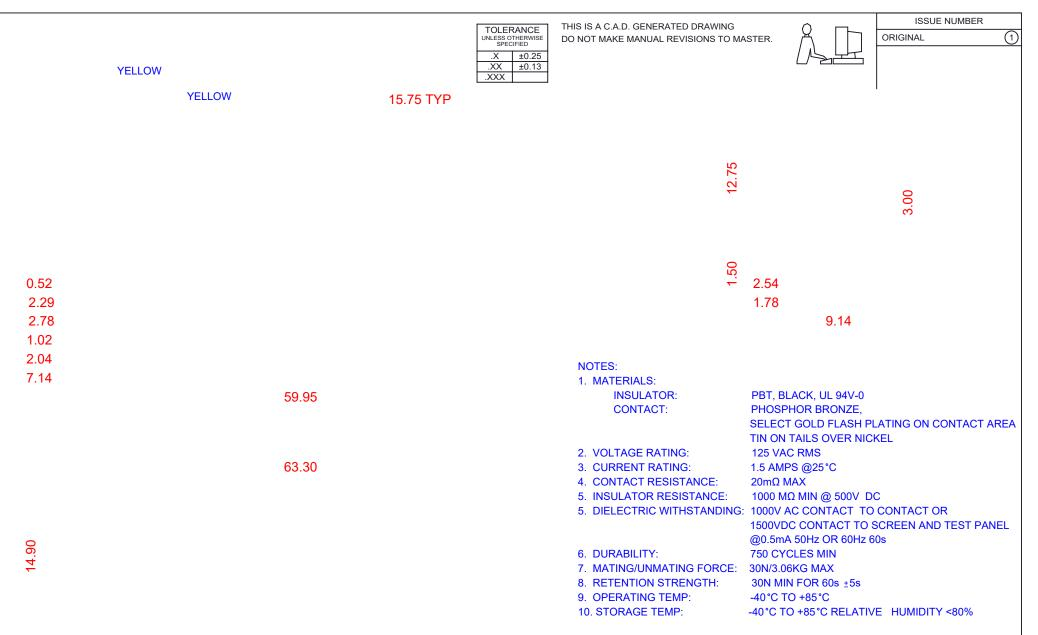
MATES WITH MODULAR PLUG CONFORMING TO FCC PART 68, SUBPART F.
