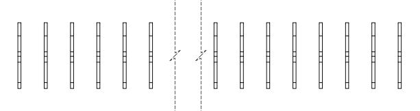
NOTE: CONTACTS ARE HELD IN A CARRIER FOR EASE OF ASSEMBLY
