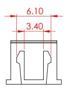
**SPECIFICATIONS VOLTAGE RATING:** 250V AC/DC 3A AC/DC **CURRENT RATING:** WITHSTANDING VOLTAGE: 1000V AC/MIN -40° C TO 105° C **TEMPERATURE RANGE: INSULATION RESISTANCE:**  $1000M\Omega$  MIN.
