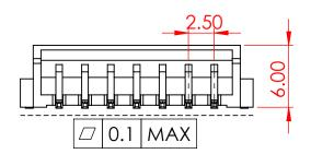
**SPECIFICATIONS VOLTAGE RATING:** 250V AC/DC **CURRENT RATING:** 3A AC/DC WITHSTANDING VOLTAGE: 1000V AC/MIN
