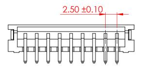
**SPECIFICATIONS VOLTAGE RATING:** 250V AC/DC **CURRENT RATING:** 3A AC/DC WITHSTANDING VOLTAGE: 1000V AC/MIN TEMPERATURE RANGE: -40°C TO 105°C TEMPERATURE RANGE: **INSULATION RESISTANCE:**  $\geq 1000 M\Omega$
