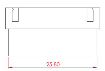
**SPECIFICATIONS VOLTAGE RATING:** 250V AC/DC 3A AC/DC **CURRENT RATING:** WITHSTANDING VOLTAGE: 1000V AC/MIN -40° C TO 105° C **TEMPERATURE RANGE: INSULATION RESISTANCE:**  $1000M\Omega$  MIN.
