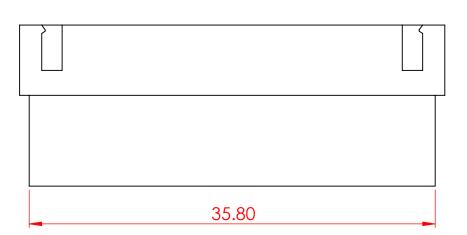
**SPECIFICATIONS VOLTAGE RATING:** 250V AC/DC 3A AC/DC **CURRENT RATING:** WITHSTANDING VOLTAGE: 1000V AC/MIN -40° C TO 105° C **TEMPERATURE RANGE: INSULATION RESISTANCE:**  $1000M\Omega$  MIN.
