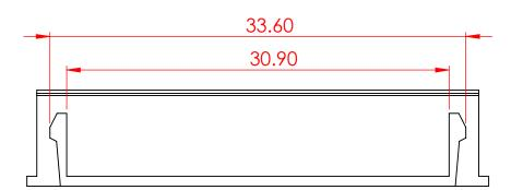
**SPECIFICATIONS VOLTAGE RATING:** 250V AC/DC **CURRENT RATING:** 3A AC/DC WITHSTANDING VOLTAGE: 1000V AC/MIN -40° C TO 105° C **TEMPERATURE RANGE: INSULATION RESISTANCE:**  $1000M\Omega$  MIN.
