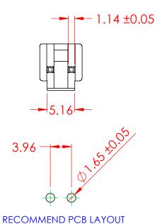
**SPECIFICATIONS VOLTAGE RATING:** 250V AC/DC 7A AC/DC **CURRENT RATING:** WITHSTANDING VOLTAGE: 1500VAC/MIN **TEMPERATURE RANGE:** -40 °C TO 105 °C **INSULATION RESISTANCE:**  $1000M\Omega$  MIN **CONTACT RESISTANCE:**  $10m\Omega$  MAX
