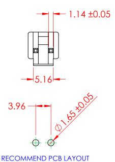
**SPECIFICATIONS VOLTAGE RATING:** 250V AC/DC 7A AC/DC **CURRENT RATING:** WITHSTANDING VOLTAGE: 1500VAC/MIN **TEMPERATURE RANGE:** -40°C TO 105°C **INSULATION RESISTANCE:**  $1000M\Omega$  MIN **CONTACT RESISTANCE:** 10mΩ MAX
