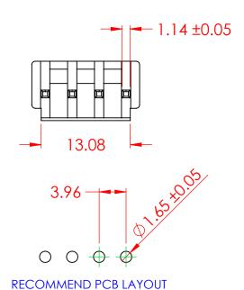
**SPECIFICATIONS VOLTAGE RATING:** 250V AC/DC 7A AC/DC **CURRENT RATING:** WITHSTANDING VOLTAGE: 1500VAC/MIN **TEMPERATURE RANGE:** -40°C TO 105°C **INSULATION RESISTANCE:**  $1000M\Omega$  MIN **CONTACT RESISTANCE:** 10mΩ MAX
