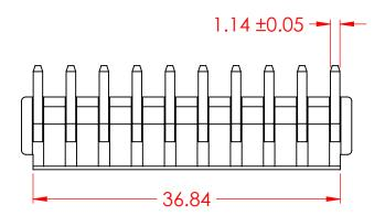
**SPECIFICATIONS VOLTAGE RATING:** 250V AC/DC 7A AC/DC **CURRENT RATING:** WITHSTANDING VOLTAGE: 1500VAC/MIN **TEMPERATURE RANGE:** -40°C TO 105°C **INSULATION RESISTANCE:**  $1000M\Omega$  MIN **CONTACT RESISTANCE:** 10mΩ MAX
