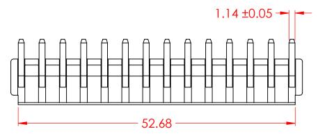
**SPECIFICATIONS VOLTAGE RATING:** 250V AC/DC 7A AC/DC **CURRENT RATING:** WITHSTANDING VOLTAGE: 1500VAC/MIN -40°C TO 105°C **TEMPERATURE RANGE: INSULATION RESISTANCE:**  $1000M\Omega$  MIN **CONTACT RESISTANCE:** 10mΩ MAX
