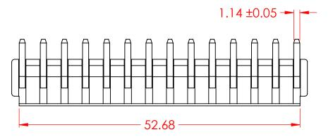
**SPECIFICATIONS VOLTAGE RATING:** 250V AC/DC 7A AC/DC **CURRENT RATING:** WITHSTANDING VOLTAGE: 1500VAC/MIN -40°C TO 105°C **TEMPERATURE RANGE: INSULATION RESISTANCE:**  $1000M\Omega$  MIN **CONTACT RESISTANCE:** 10mΩ MAX
