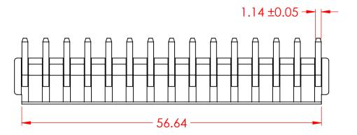
**SPECIFICATIONS VOLTAGE RATING:** 250V AC/DC 7A AC/DC **CURRENT RATING:** WITHSTANDING VOLTAGE: 1500VAC/MIN -40°C TO 105°C **TEMPERATURE RANGE: INSULATION RESISTANCE:**  $1000M\Omega$  MIN **CONTACT RESISTANCE:** 10mΩ MAX
