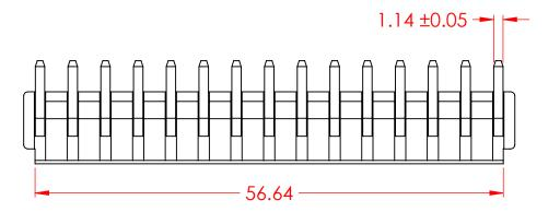
**SPECIFICATIONS VOLTAGE RATING:** 250V AC/DC 7A AC/DC **CURRENT RATING:** WITHSTANDING VOLTAGE: 1500VAC/MIN -40°C TO 105°C **TEMPERATURE RANGE: INSULATION RESISTANCE:** 1000ΜΩ ΜΙΝ **CONTACT RESISTANCE:** 10mΩ MAX
