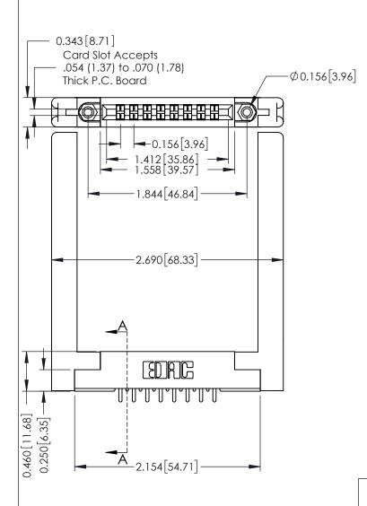
0.295 [7.49] Card Slot 0.165[4.19] Point of Contact 306 / 316 / 356 Card Edge Connector Part Number: 306-008-521-158
