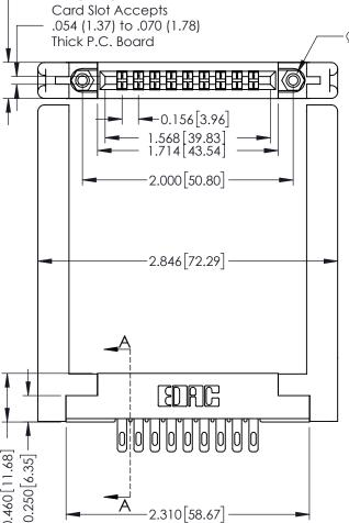
A-A SECTION 0.295 [7.49] Card Slot 0.165[4.19] Point of Contact
