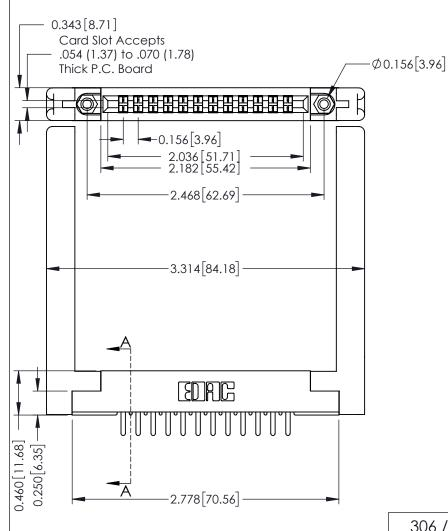
SECTION 0.295 [7.49] Card Slot 0.165[4.19] Point of Contact
