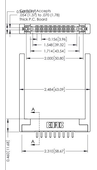
A-A0.295[7.49] Card Slot **ECTION** 0.090[2.29] Point of Contact 305 ENG MASTER 305 / 315 / 355 Card Edge Connector
