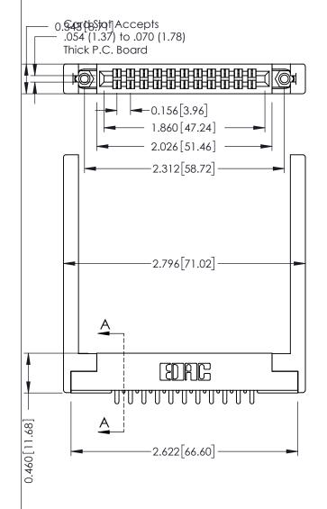
SECTION A-A 0.295[7.49] Card Slot 0.090[2.29] Point of Contact
