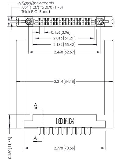
SECTION A-A 0.295[7.49] Card Slot 0.090 [2.29] Point of Contact
