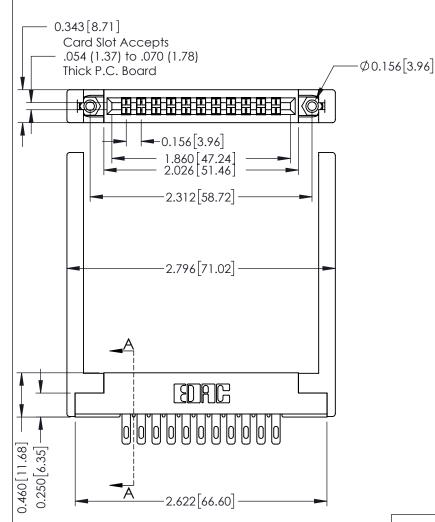
SECTION A-A 0.295 [7.49] Card Slot 0.165[4.19] Point of Contact
