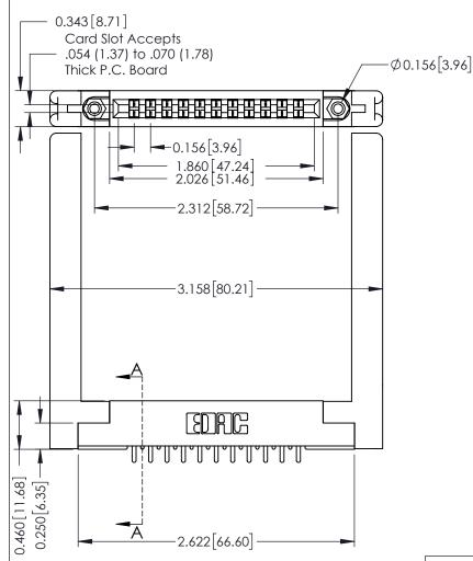
A-ASECTION 0.295 [7.49] Card Slot 0.165[4.19] Point of Contact
