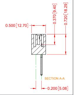
ACAD REFERENCE NO .: 317 Assembly **317 SERIES CARD EDGE CONNECTOR** DATE: February 5, 2020 DRAWN: C.B CHECKED: DATE: THESE DRAWINGS AND SPECIFICATIONS OF SCALE: 1:1 SHEET 1 1 EDAC INC ARE THE PROPERTY OF EDAC INC..AND TORONTO, ONTARIO SHALL NOT BE REPRODUCED, OR COPIED 317-024-542-601 DRAWING NUMBER: ISSUE OR USED AS THE BASIS FOR THE CANADA MANUFACTURE OR SALE OF APPARATUS 1 YOUR CONNECTION TO QUALITY & SERVICE PART NUMBER: 317-024-542-601 WITHOUT WRITTEN PERMISSION.
