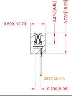
ACAD REFERENCE NO .: 317 Assembly 317 SERIES CARD EDGE CONNECTOR DATE: February 5, 2020 DRAWN: C.B CHECKED: DATE: THESE DRAWINGS AND SPECIFICATIONS OF SCALE: 1:1 SHEET 1 1 EDAC INC ARE THE PROPERTY OF EDAC INC..AND TORONTO, ONTARIO SHALL NOT BE REPRODUCED, OR COPIED 317-028-541-602 DRAWING NUMBER: ISSUE OR USED AS THE BASIS FOR THE CANADA MANUFACTURE OR SALE OF APPARATUS 1 YOUR CONNECTION TO QUALITY & SERVICE PART NUMBER: 317-028-541-602 WITHOUT WRITTEN PERMISSION.
