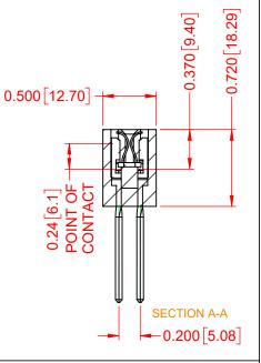
ACAD REFERENCE NO .: 317 Assembly 317 SERIES CARD EDGE CONNECTOR DATE: February 5, 2020 DRAWN: C.B CHECKED: DATE: THESE DRAWINGS AND SPECIFICATIONS OF SCALE: 1:1 SHEET 1 1 EDAC INC ARE THE PROPERTY OF EDAC INC..AND TORONTO, ONTARIO SHALL NOT BE REPRODUCED, OR COPIED 317-068-543-808 DRAWING NUMBER: ISSUE OR USED AS THE BASIS FOR THE CANADA MANUFACTURE OR SALE OF APPARATUS 1 YOUR CONNECTION TO QUALITY & SERVICE PART NUMBER: 317-068-543-808 WITHOUT WRITTEN PERMISSION.
