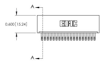
0.600[15.24] SLOT DEPTH 0.127[3.23] POINT OF CONTACT **SECTION A-A**
