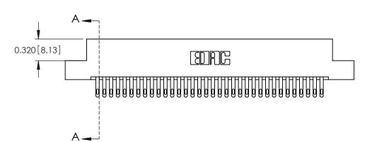
0.600[15.24] 0.297 7.54 SLOT DEPTH 0.127[3.23] POINT OF CONTACT **SECTION A-A**
