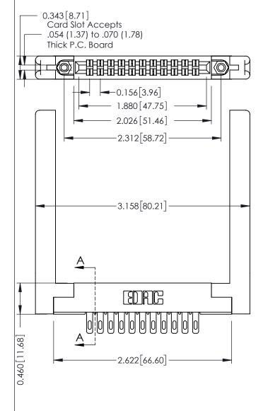
0.295[7.49] Card Slot ECTION 0.090 [2.29] Point of Contact 305 ENG MASTER 305 / 315 / 355 Card Edge Connector
