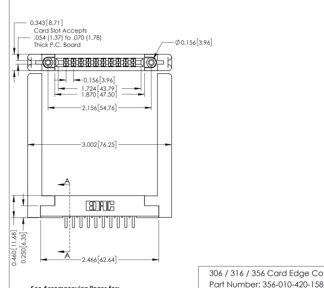
SECTION 0.295 [7.49] Card Slot 0.165[4.19] Point of Contact ACAD REFERENCE NO. 306 ENG MASTER 306 / 316 / 356 Card Edge Connector
