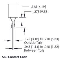
379 Series Card Edge Connector Contact Bend Detail
