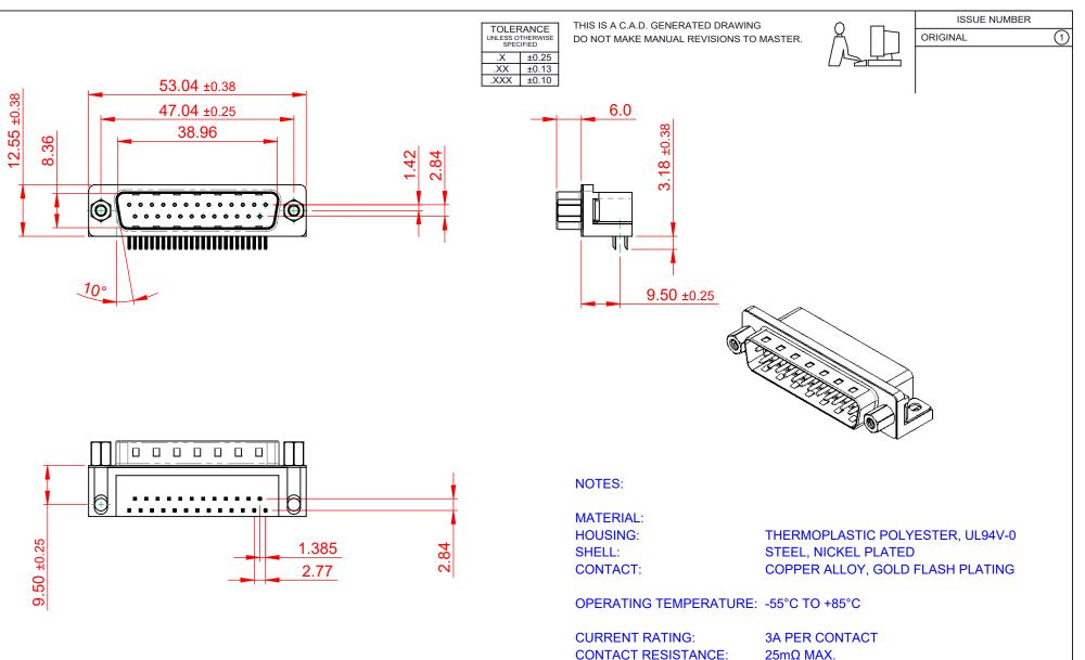
DIELECTRIC WITHSTANDING VOLTAGE: 1000V AC rms
