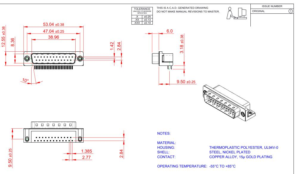
**CURRENT RATING:** CONTACT RESISTANCE: **INSULATOR RESISTANCE:** DIELECTRIC WITHSTANDING VOLTAGE: 1000V AC rms
