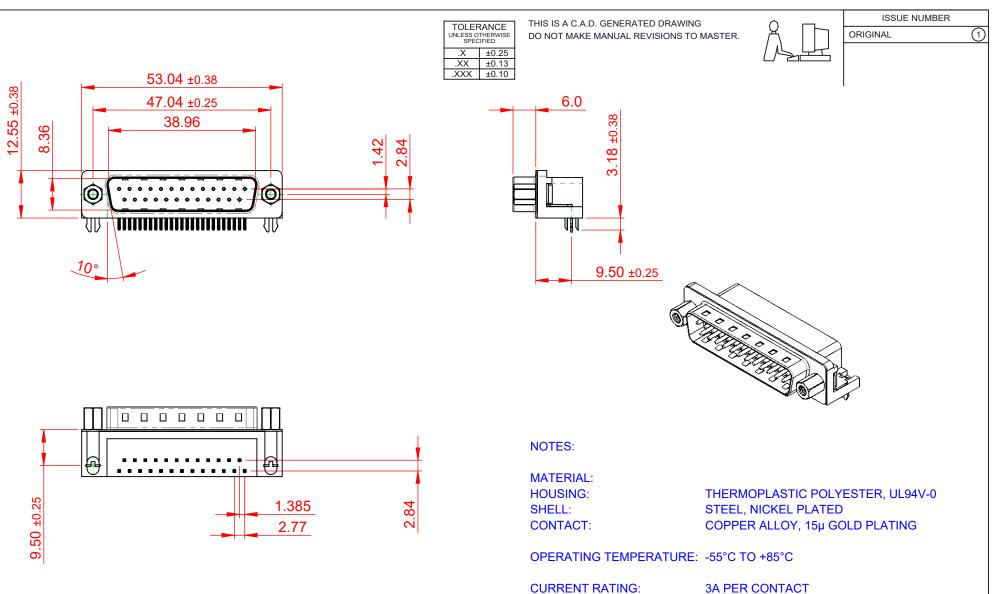
CONTACT RESISTANCE: **INSULATOR RESISTANCE:** DIELECTRIC WITHSTANDING VOLTAGE: 1000V AC rms
