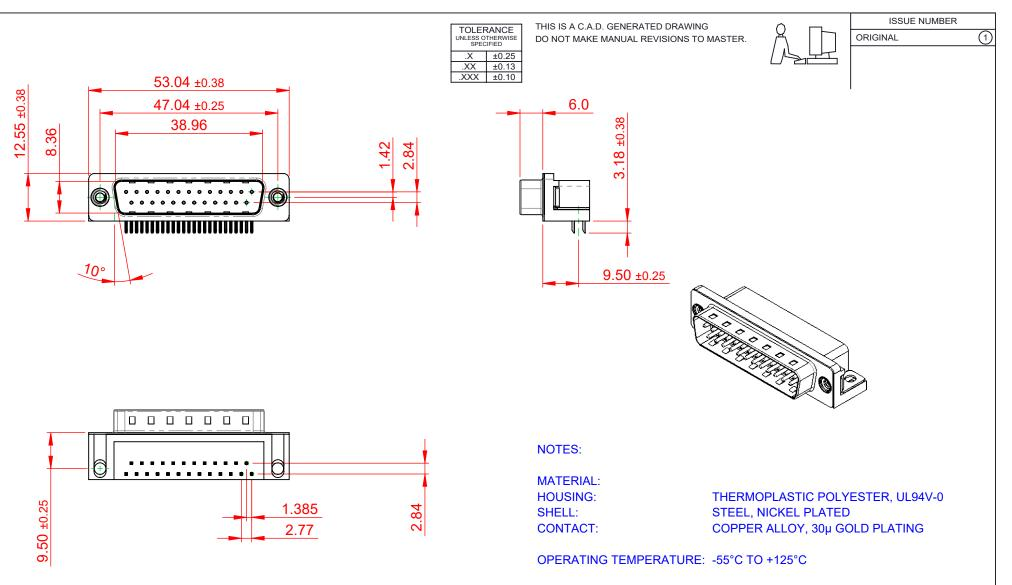
CURRENT RATING: CONTACT RESISTANCE: **INSULATOR RESISTANCE:** DIELECTRIC WITHSTANDING VOLTAGE: **3A PER CONTACT** 25mΩ MAX.
