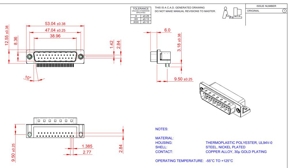
CURRENT RATING: CONTACT RESISTANCE: **INSULATOR RESISTANCE:** DIELECTRIC WITHSTANDING VOLTAGE: **3A PER CONTACT** 25mΩ MAX. 5000MΩ min.
