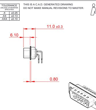
MATERIAL: HOUSING: PA6T, UL94V-0 SHELL: STEEL, Sn or Ni PLATED CONTACT: PRECISION MACHINED COPPER ALLOY SEE ORDERING GUIDE FOR CONTACT PLATING
